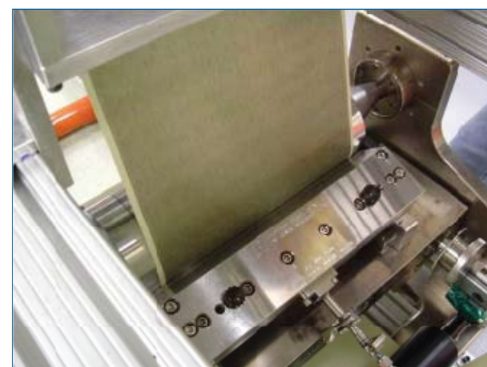
CNK ink deposited on flexible plastic film using slot die coater at Chasm Technologies.
